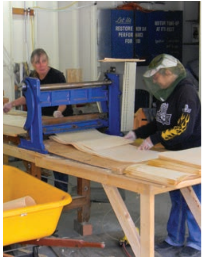
Cutting and stacking veneer
